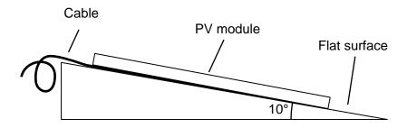
Figure 3. Side view of module prepared for testing.
