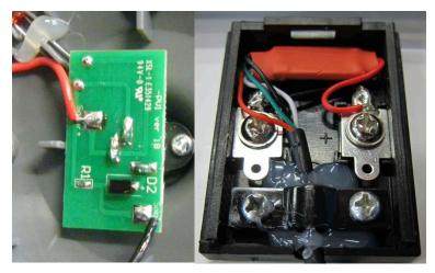
Figure 1. Examples of DUTs containing "a circuit board or other sensitive electronics" and requiring water ingress testing.
