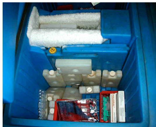
Figure 1. Example of a vaccine transport container with ice packs or cool water-packs designed to maintain 2-8°C for over 12 hours ©GiveWell
