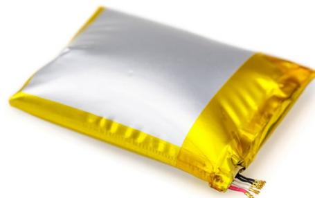
**Figure 9. Swelling of a Li-ion pouch cell**
