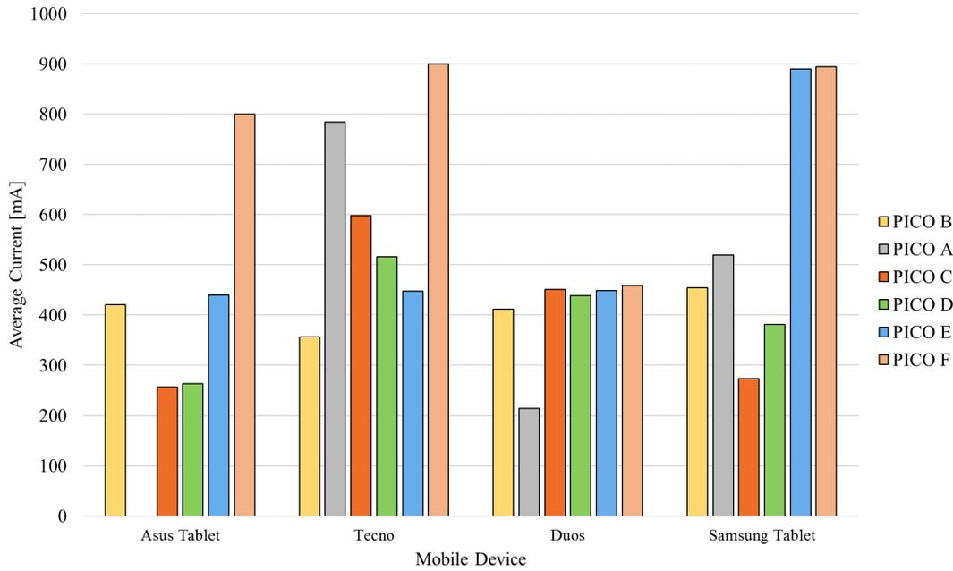
FIGURE 5: ERRATIC CHARGING BEHAVIOR FOR PICO B AND TECHNO Y2 PRODUCT COMBINATIO
