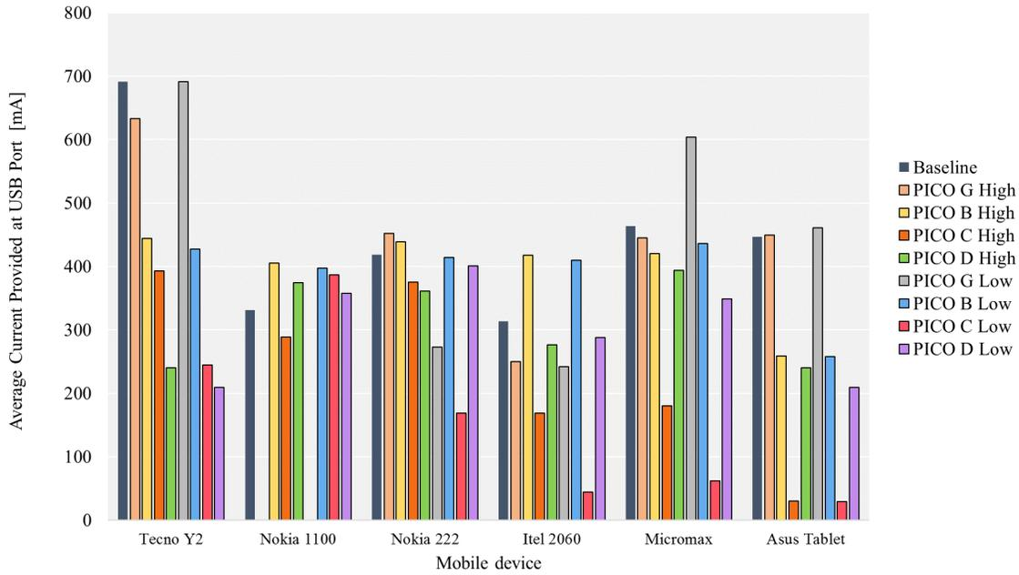
FIGURE 12: AVERAGE OFF-GRID PRODUCT CHARGING EFFICIENCY
