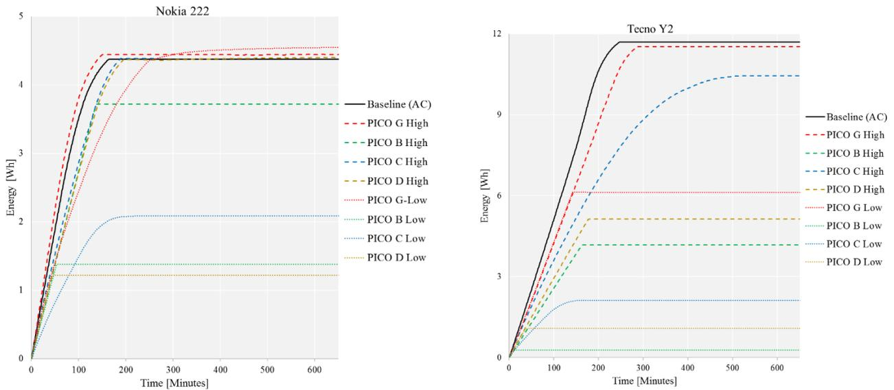
FIGURE 10 (CONT): ENERGY ACCUMULATED BY MOBILE DEVICES DURING PHASE III TESTING
