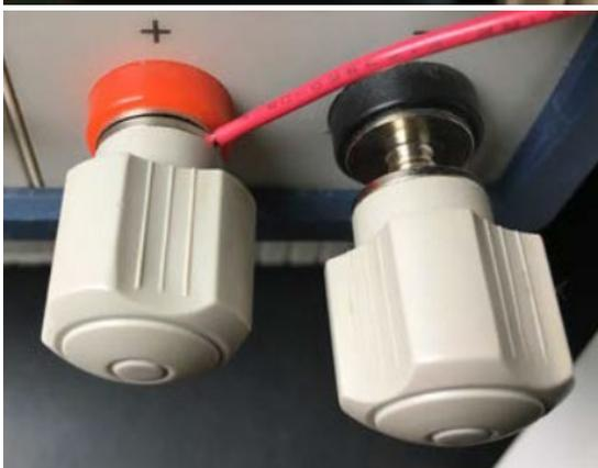
Some binding posts may have a hole to insert the wire; in others, the wire needs to be wrapped around the post. *Only those that have holes to insert the wire are permitted. Those that require wrapping the wire are not permitted due to the increased likelihood of the connection being improperly made.* No tools except wire strippers are required.
