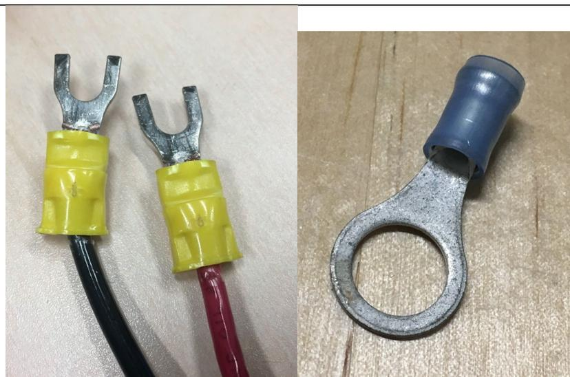
These connections can be more secure than those made with bare wire, but the installer must be trained in proper crimping technique and the tool, terminal, and wire size must all be matched, or a poor connection will result. In addition, training is needed to distinguish a good crimp from a poor crimp.
