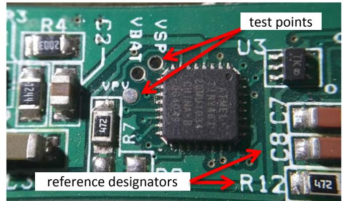
Figure 2. circuit board silkscreen labels
