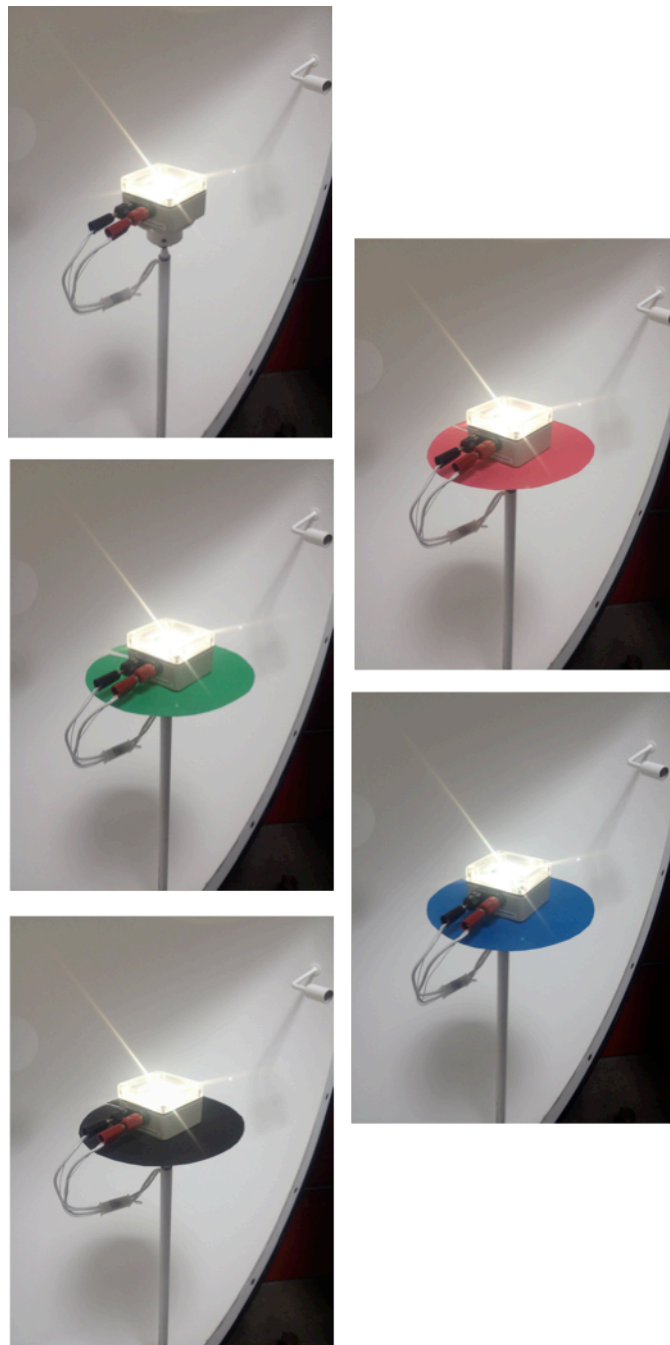
Figure 2. An experiment to check the AUX correction accuracy of an integrating sphere system. The input flux from the LED light source remains constant while the sphere throughput changes with different colored sheets of paper. Proper AUX correction can account for these changes.
