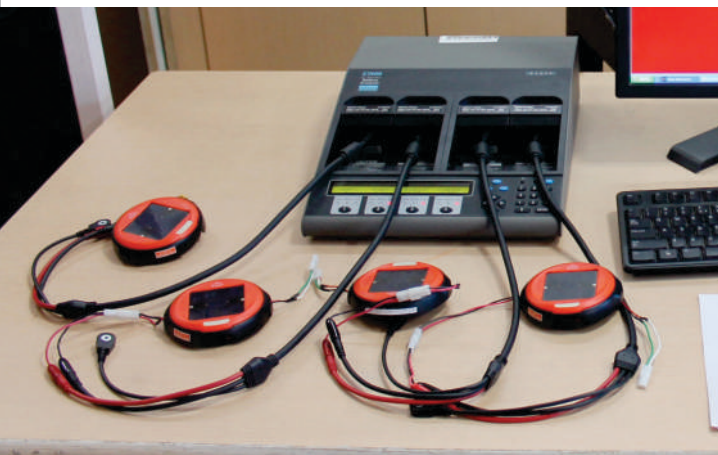
Equipment-Battery capacity test bench
