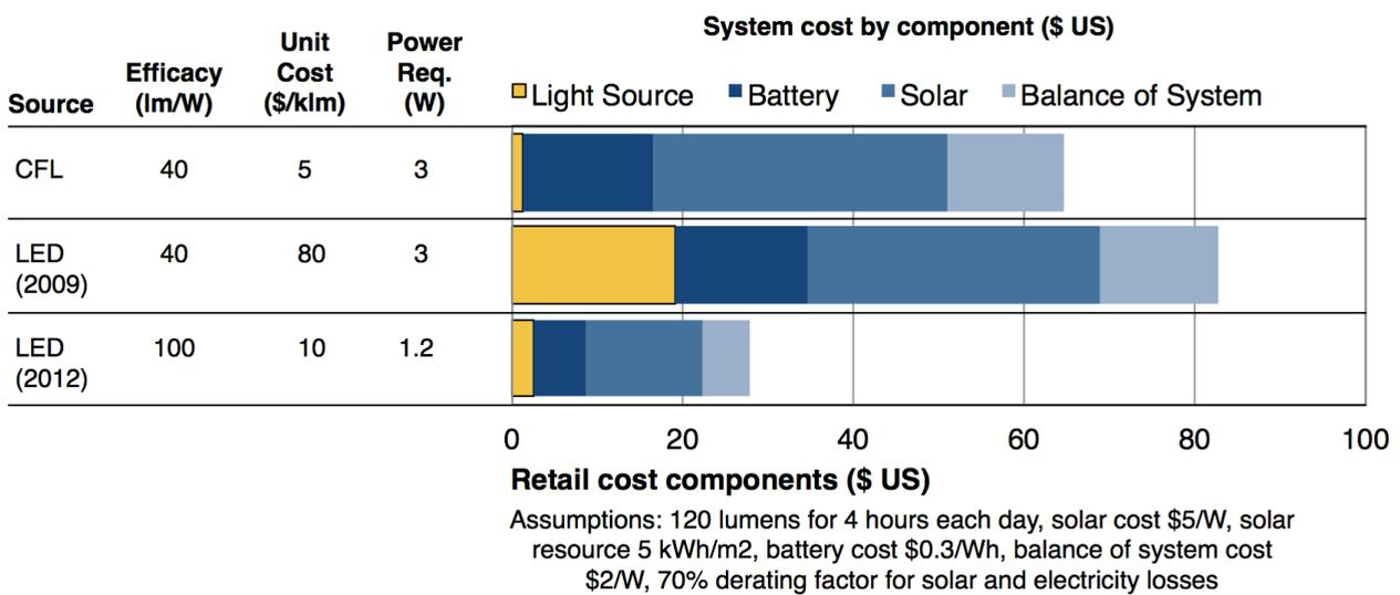
**Figure 3:** Estimated cost for generic, high performance LED and CFL products. The energy side performance and cost for each system is fixed so the model shows the relationship between light source cost and performance and assembled system cost.
