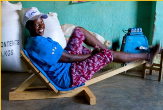
The Nuru Light is pedal-powered © John Briggs
