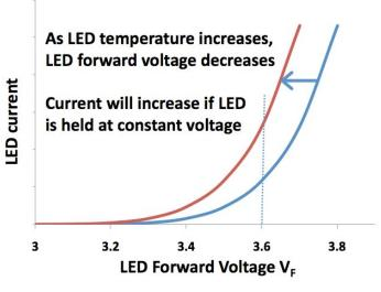
Figure 1. LED thermal runaway
