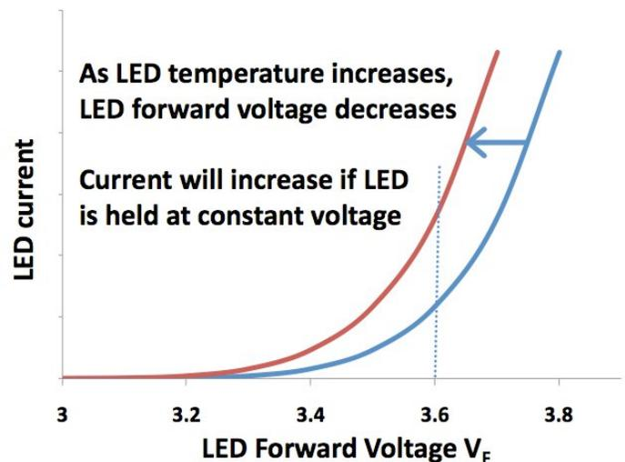
Figure 1. LED thermal runaway
