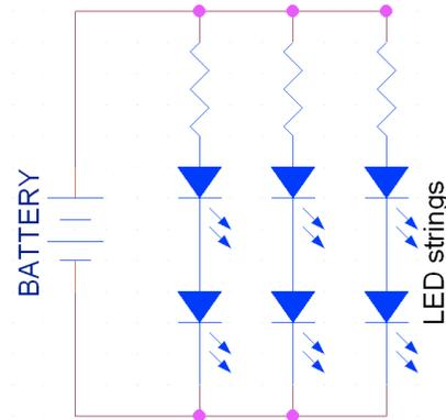
Figure 4. Series/Parallel LED Array with Current Balancing Resistors
