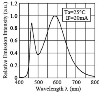
**Graphs** provide much of the data necessary to run the LED in a safe, reliable manner. The examples shown here should all be included *somewhere* in the datasheet, though the format and presentation may be different.
