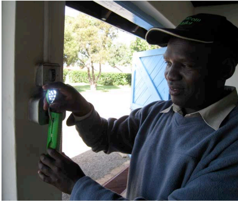
Figure 9: A torch / task light hybrid product, being shown to us by a worker at a Unilever guesthouse near Kericho. It is currently being charged using AC grid electricity. He is extending a task light head from its cradle in the handle of a torch. It is a common product that can be found in town. Note that there is no feature preventing the lamp from being switched on during charging.
