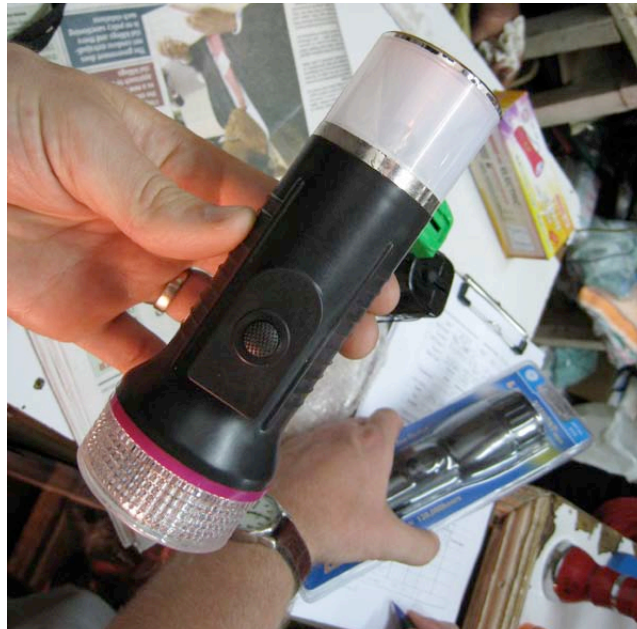
Figure 10: A torch / ambient light hybrid product, available in Kericho. The ambient lighting is achieved by a conical mirror (visible on top) which scatters the light of upward-facing LEDs.
