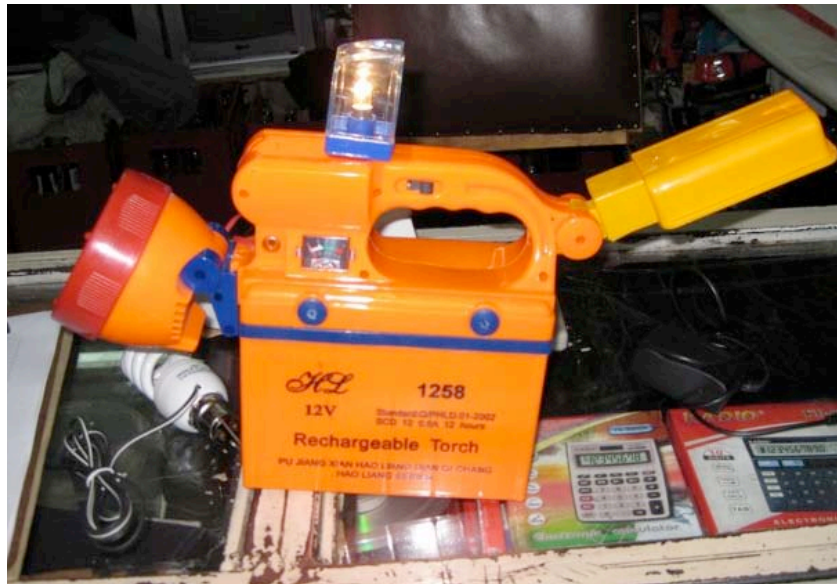
Figure 11: A combination torch / task / ambient light that we observed in Kericho with an unusual design; it has an LED "spotlight", a fold out array of LEDs, for task lighting, and an incandescent bulb on top for ambient lighting. The light is powered by a somewhat large 12 V sealed lead acid battery that includes an indicator gauge for the voltage (state of charge).
