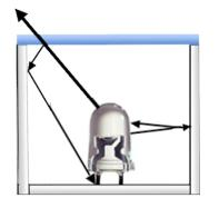
Figure 9. A constrained optical cavity. Light leaving the LED can get selfabsorbed or trapped in small corners.
