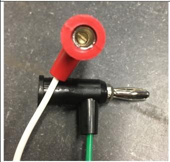
Only connectors with attachment mechanisms similar to those described above (wire is inserted into a hole and clamped down, binding posts, etc.) are considered acceptable. In the picture to the left, wire is inserted in the hole in the bottom of the plug and a set screw in the back of the plug is tightened to hold the wire in place.
