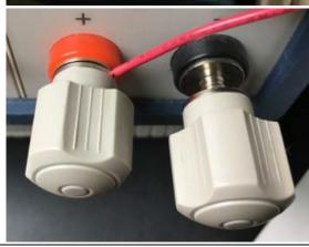
Some binding posts may have a hole to insert the wire; in others, the wire needs to be wrapped around the post. Only those that have holes to insert the wire are permitted. Those that require wrapping the wire are not permitted due to the increased likelihood of the connection being improperly made. No tools except wire strippers are required.
