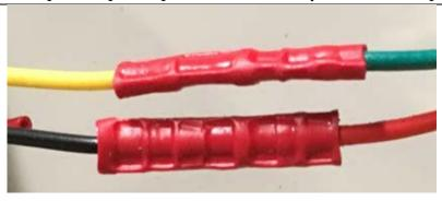
These connections require skill and the proper tools to install correctly.
