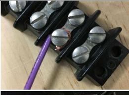
It is easy to fail to secure all the strands in this connection, which can increase the resistance of the connection or short with neighboring terminals.
