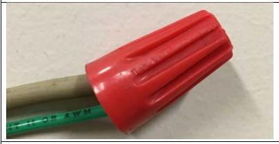
These are very common in building wiring in some countries (including the US) and uncommon in others (such as the UK). They are not suitable for wires that are subject to flexing or pulling (unless strain relief is provided) and are not suitable for outdoor use.
