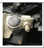
The wire must be either terminated at the factory or connected using one of the other acceptable methods listed in this document (such as clamped between two plates).
