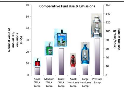
Fig. 3 Rates of fuel use vary widely among lamps. Those shown in this figure vary from 0.018 to 0.089 l of kerosene per hour. Annual estimates are based on 4-h/day use, a 5-year time horizon, an emissions factor of 2.4 kg  $CO_2/l$ , and an illustrative emissions price of \$20/ton  $CO_2$ . Note that the vast preponder-
