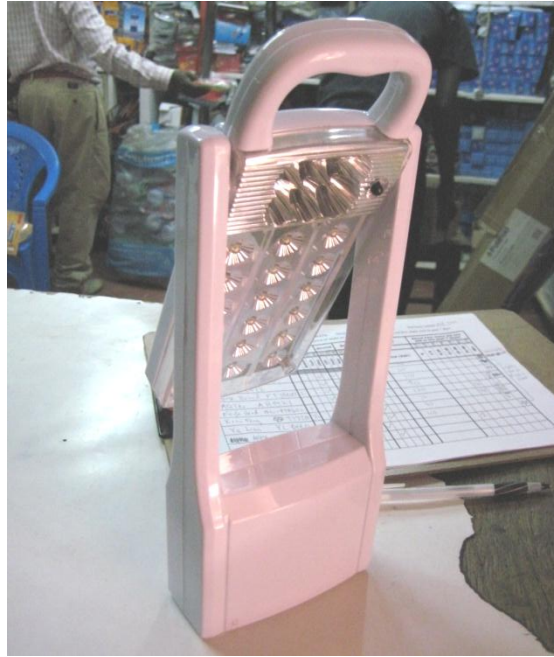
Figure 12: An ambient / task light hybrid product. Large LED arrays such as these were common in Kericho and typically marketed as emergency lights.
